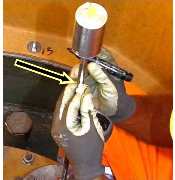
Mark the "Safety Distance" 10 mm below, press the probe down to this point
