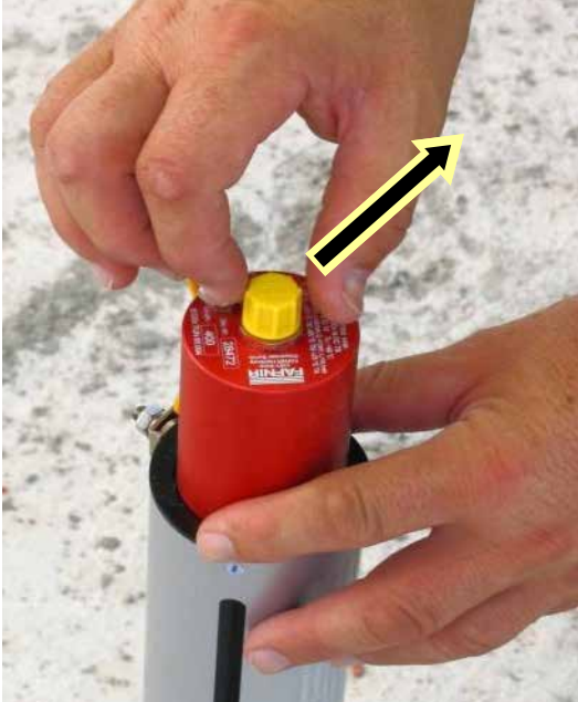
Unscrew yellow cap and connect the plug
