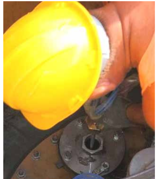
Insert probe until bottom is reached
