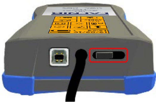
Figure 28: Switch in USB position (charging position)
